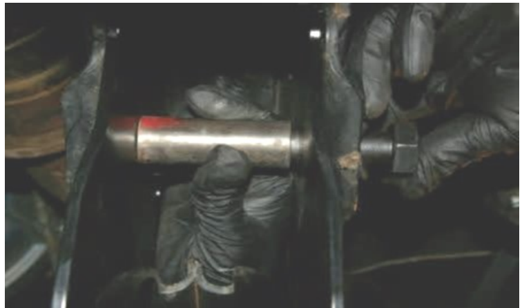
Insert crush sleeves and new hardware into drop bracket.
