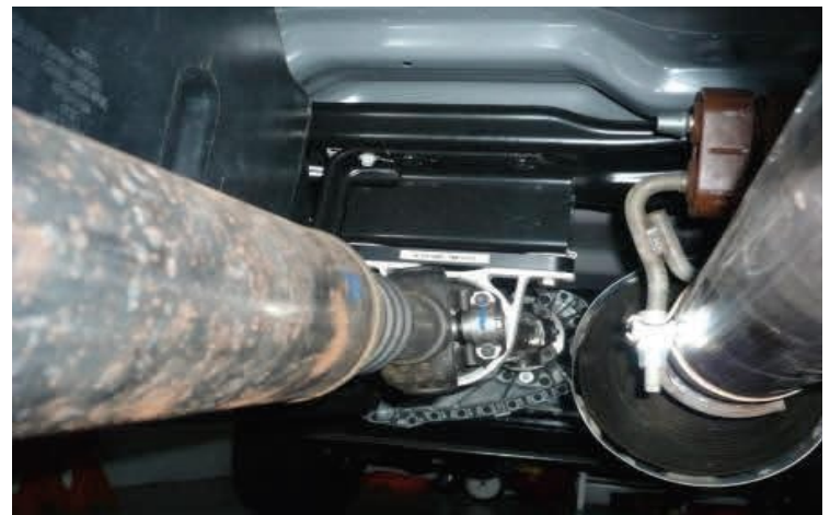
Two piece drive shaft only. With vehicle on the ground install carrier bearing drop plate.
