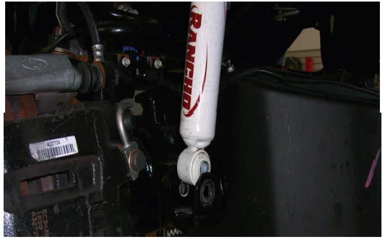
Disconnect dr./pass. front lower shock bolts
