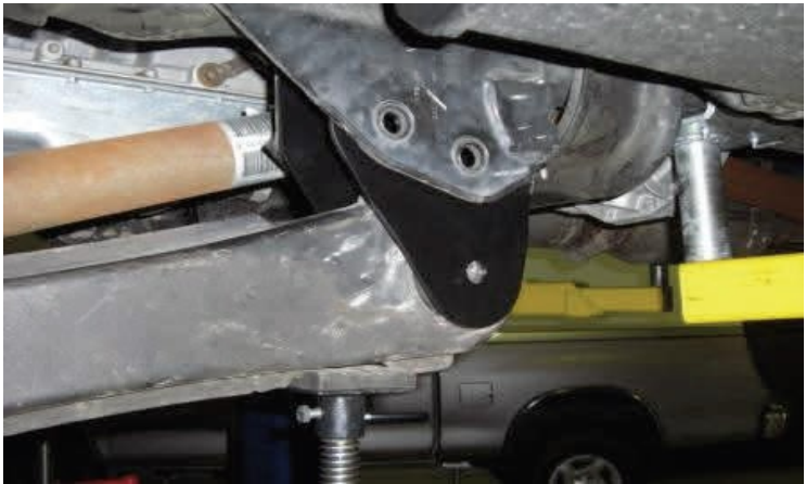
Align bracket with holes in frame and raise arm into bracket.
