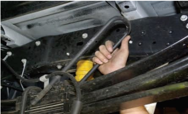
Remove U-bolts and slowly lower axle to remove OE block.
