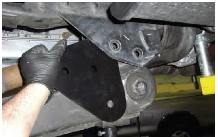
Carefully lower arm enough to slide drop bracket into frame.
