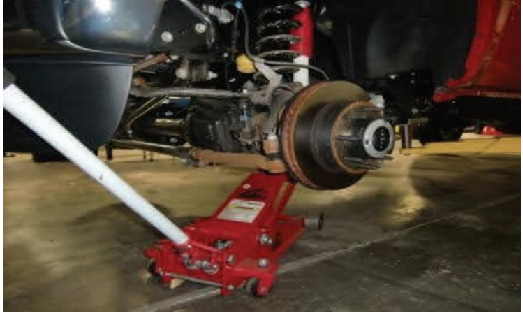
Support front axle with floor jack(s).
