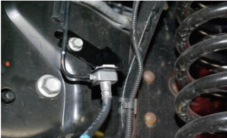
Reinstall block into bracket with retaining clip.
