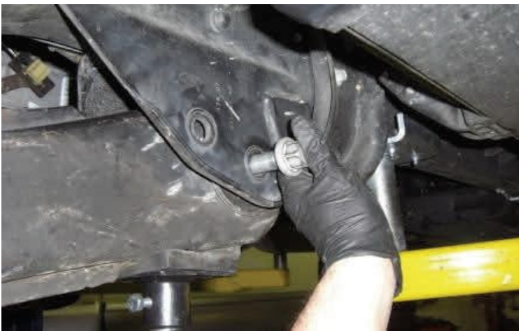
Support radius arm and remove attachment bolts
