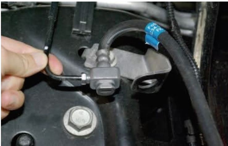
Loosen hard line ferrule rotate block 180 degrees and tighten
