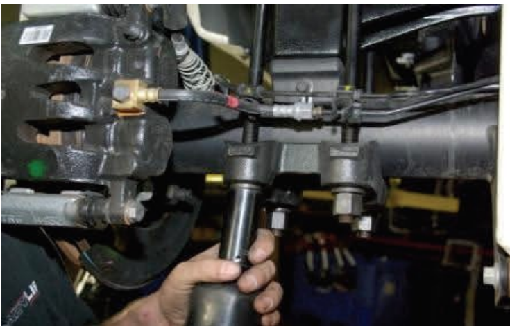
Install longer U-bolts and nuts onto axle plate. Torque later.
