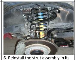
stock location. Leave the three upper strut mounting nuts loose Raise the lower control arm and install the lower strut mounting bolt and nut. Use a floor jack to raise the lower control arm up in order to get the lower ball joint bolts installed. Be sure to use a thread locker on the lower ball joint bolts.
