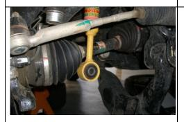
**4**. Remove the lower strut mount nut and bolt. Push the lower control arm down.
