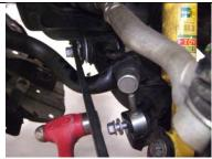
Use of a pry bar and hammer may be need to align mounting holes for the end link bolt. Install 19mm bolt and torque to factory specs.
