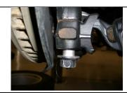
Loosen and remove the two 22mm bolts that connect the lower ball joint to the spindle. Please take caution as the lower control arm will swing down as soon as you remove the lower ball joint bolts. Holding the Strut with one
