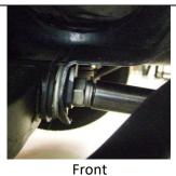
Using a 24mm socket, loosen but don't remove the driver side lower control arm bolts. This will allow the lower control arm to move freely.
