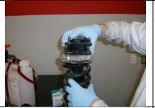
Install the TrailFx strut extension and torque to factory specs.
