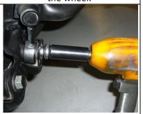
Using a 19mm socket, loosen and remove the sway bar end link bolt on the lower control arm.
