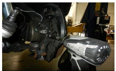
Remove the cotter pin and outer tie rod end nut. Strike the tie rod end boss with a dead blow hammer to dislodge the taper. Remove the ABS sensor and harness from the knuckle and hang out of the way.
