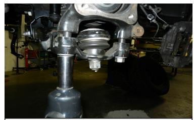
Remove the lower strut bolt. Remove the ball joint cradle bolts and let lower control arm swing out of the way. Remove the strut from the vehicle.
