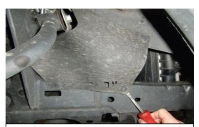
Remove the front splash guards from the frame for access to the upper control arm bolt.
