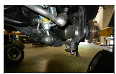
Remove the sway bar from the lower control arm. Loosen the lower control arm bolts.
