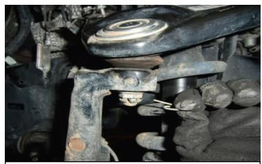
Remove the upper ball joint safety clip and nut. Strike the ball joint boss with a dead blow hammer to dislodge the taper.
