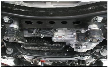
Remove the front diff mount to frame bolts. Lower the diff low enough to insert the provided diff spacers. Install using the provided longer hardware.
