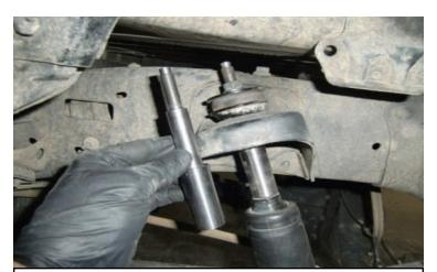
Install the provided shock extensions to the shock. Install the shock back to the vehicle using the factory hardware. Install the brake line brackets back to the axle. Make sure everything is torqued down and there is clearance for the tires against all moving parts. Have the alignment set.
