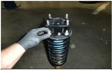
Install the strut extension to the strut using the factory hardware. Install the completed strut into the frame using the provided hardware. Raise the lower control arm to the strut and install the factory hardware. Install the lower ball joint cradle to the knuckle using the factory hardware.
