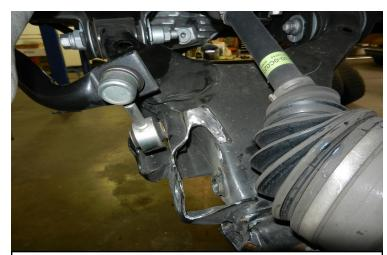
Notch the lower control arm strut pocket as shown using a suitable cutting device. Sand any burs off the cut edge. Paint the cut area with a quality rust preventative paint.
