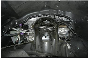
Remove the upper control arm from the frame. (Strut shown removed for clarification. Will be removed in a later step.)
