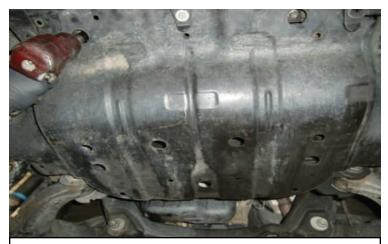
4WD steps: Remove the factory skid plate.
