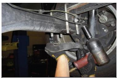
Remove the u bolts on the side you intend to work on first. Lower the axle low enough to insert the provided lift blocks. Install the provided u-bolts and axle cradle. Repeat for the other side of the vehicle.
