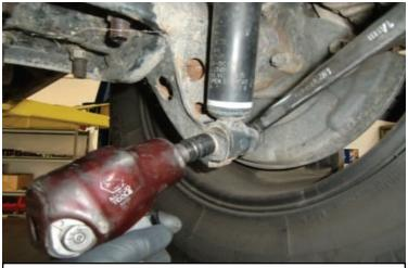
Support the rear axle. Remove the rear shocks, brake line brackets, and parking brake cable brackets from the axle.
