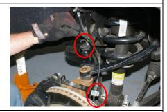
4. A 10mm socket is used to remove the brake line bracket that attaches to the upper control arm.
