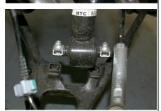
10. Remove the three upper strut nuts that secure the strut to the frame housing.
