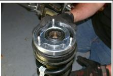
13. Carefully install the strut with the ReadyLift spacer on top into the upper frame pocket. Secure the strut with the provided new nuts. Leave the nuts only hand tight so the bottom of the strut can be adjusted when the lower control arm is raised up.
