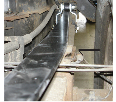
SuperSprings installed on top of factory block.
