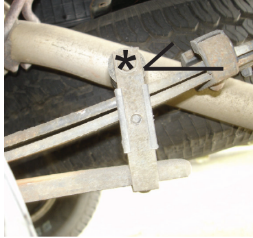
Remove bolt and roller from the rear rebound bracket. Do not remove bracket.
