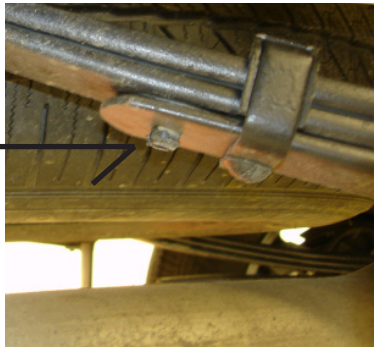
Use a chisel to trim off plastic tab. Ensure the plastic tab is flush with the bottom of the factory spring.
