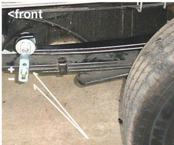
Adjustable pre-load and ride height [fnt/rear]
