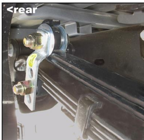
front & rear ~ adjustable preload
