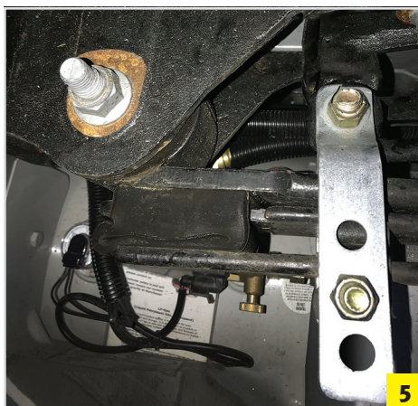
On vehicles with CAST steel leaf spring mounts: the middle hole of the SSA43 shackle MUST be used.
