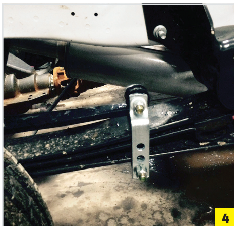
On vehicles with STAMPED steel leaf spring mounts: either the lower or middle hole of the SSA43 shackle may be used.
