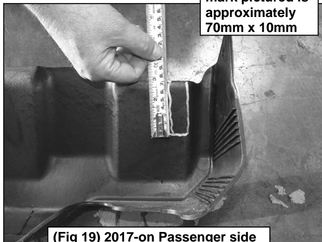
(Fig 19) 2017-on Passenger side DEF cover marked for trimming
