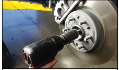
Remove the axle nut from the hub.
