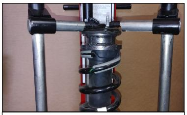
Place strut in a spring compressor. Remove factory top hat. Install in between the top hat with rubber isolator and the factory plastic spring mount.
