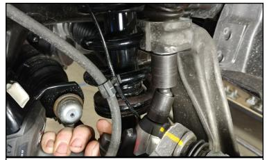
Remove the upper ball joint from the knuckle. Let knuckle hang out of the way. Do not stretch the ABS/ brake lines.
