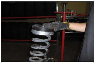
Lower the control arm down to remove the spring. Install the spring spacer on top of the spring. Install into the frame and raise the lower control arm back up to install the arm hardware. Reverse the rest of the disassembly steps. Have the vehicle aligned.
