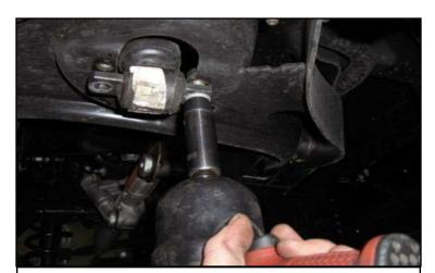
Support the lower control arm at the knuckle. Remove the lower shock hardware.
