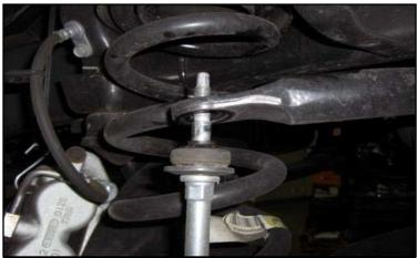
Raise vehicle. Remove front wheels. Remove the sway bar end links from the sway bar. Push sway bar up and out of the way.
