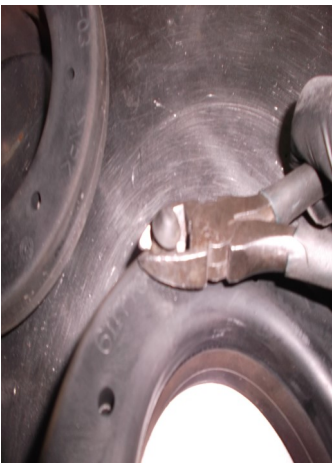
On OE spring isolator, cut off the rubber locating tab.
