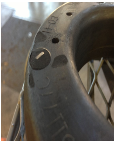
On OE spring isolator, cut off the rubber locating tab.
