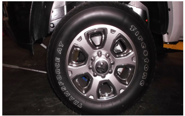
Reinstall the front wheels and put the vehicle on the ground. Torque the front wheels to factory specs.
