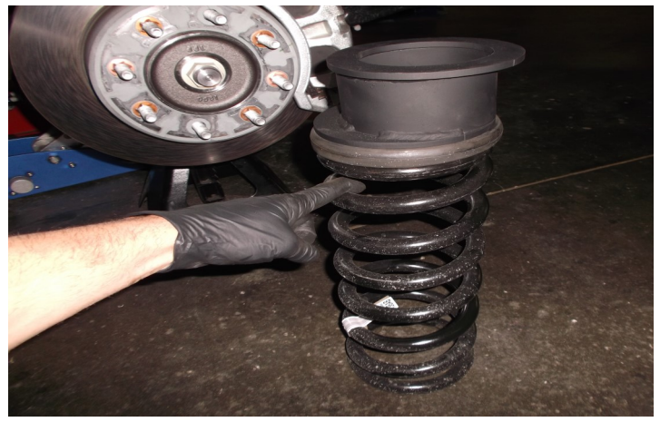
Install the OE spring isolator and the strut spacer onto the coil spring. Lower the axle further to allow spring installation.
