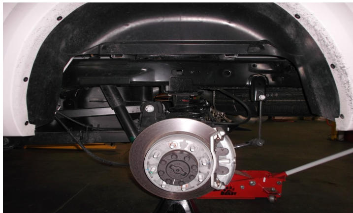
Rear Installation: Place the vehicle on level ground. Lift the vehicle by the frame, support the axle, and remove the wheels.
