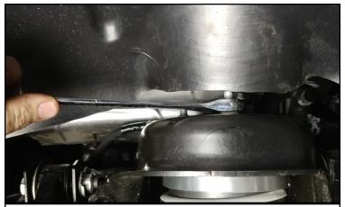
Remove the lower strut hardware. Remove the upper strut hardware. Remove the strut from the vehicle.
