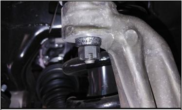
Install the upper ball joint to the knuckle using the supplied spacer and nut. Once tight, install the suppled cotter pin.
