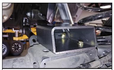
Install the bump stop extensions using the provided hardware. Utilize the holes that line up with the axle. The driver and pass sides will use different holes. Install the rear wheels and lower the vehicle to the ground.
