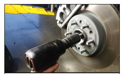
Remove the axle nut from the hub.
