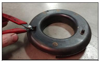
Cut off the nipples from the spring isolator.
