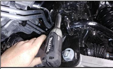
Reinstall the sway bar to the frame. Install the front wheels and lower the vehicle to the ground. Raise the rear of the vehicle. Remove the rear wheels.
