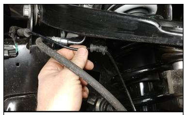
Remove the front wheels. Remove the ABS wire on the upper control arm, frame, and rubber brake line. Remove the metal brake line bracket at the frame.
