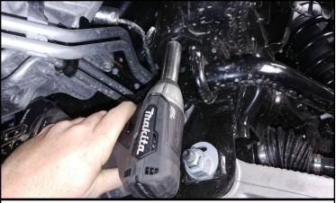
Remove the sway bar from the frame. Let hang out of the way.
