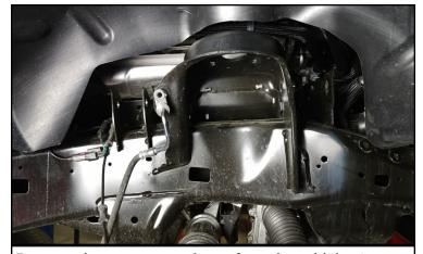
Remove the upper control arm from the vehicle. Assemble the aftermarket arms by installing the polyurethane bushings and sleeves. Use provided grease for the sleeves.
