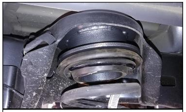
Install the spring spacer on top of the spring and isolator. Install into the frame. Raise the axle to hold everything in place. Install the lower shock, the sway bar end link, brake lines, ABS harness and any other harness that was removed.
