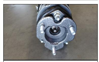
Install the strut extension to the strut using the factory nuts.
