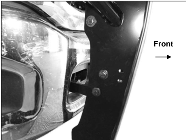
(Fig 12) Attach Grill Guard to outside of Mounting Brackets (passenger/right side pictured)
