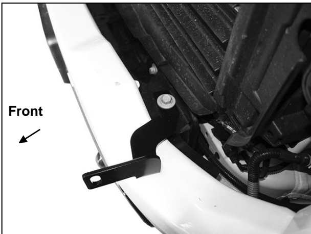
(Fig 7) Reuse bumper bracket bolt to attach driver/left Top Bracket to top of frame
