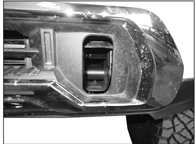
(Fig 10) Reinsert tow hook. Insert driver/left outer Frame Bracket through opening and along outside of frame
