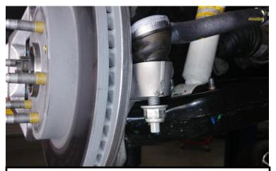
Loosen the tie rod end nut. Strike the tie rod stud with a hammer to dislodge the taper. Remove tie rod from knuckle.
