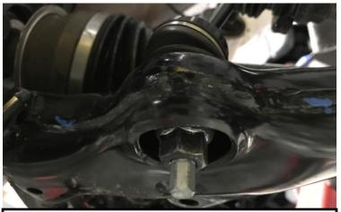
Support the lower control arm with a suitable jack. Remove the front wheels. Remove the sway bar from lower control arm and let hang.
