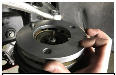
Lower the strut out of the frame. Install the tapered shim onto the strut with the thick end facing outwards. Install the upper strut using the factory hardware. Only install the back nut for now. Do not tighten all the way.
