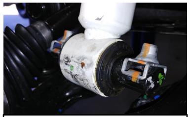
Remove factory clip nuts and discard. Supplied hardware will be used in its place. Install the lower strut spacer using the provided hardware.
