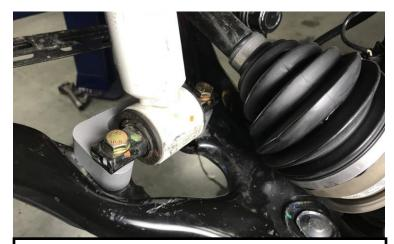
Raise the lower control arm up with the jack. You will have to load the suspension to install the upper control arm to the knuckle. Install the upper ball joint nut. Install Tie Rod end. Install Axle nut. Install the brake line bracket to the upper control arm. Install the sway bar to control arms. Install the wheels and tires. Have the alignment set.
