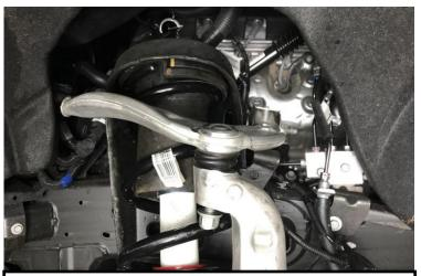
Loosen the upper ball joint nut. Strike the upper ball joint boss with a hammer to dislodge the taper. Remove Ball joint from knuckle. Remove the upper and lower strut hardware. Lower the control arm to gain clearance to remove strut.
