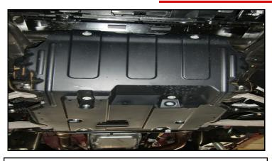
Remove the plastic gravel guard and support the front differential with a suitable jack.
