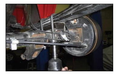
Slightly loosen but do not remove the driver side u-bolts. Remove the passenger side u-bolts completely and discard. Lower the axle enough to remove the factory lift block making sure that all brake lines and ABS lines do not get over extended.
