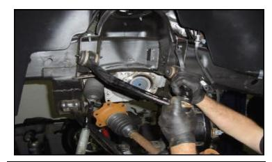
Remove the upper control arm cam bolts. Note their orientation and locations. They will need to be reinstalled the same way as removed. Remove the upper control arms from the frame.
