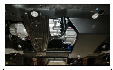
Install the provided skid plate to the frame using factory hardware. Swap the metal bracket from the passenger side of the gravel guard back to the frame. Discard the driver side. Torque to 5 ft-lbs. Make sure to not over tighten and strip out the frame holes. These are self tapping bolts.
