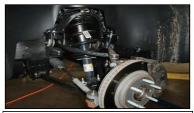
Park vehicle on a clean flat surface and block the rear wheels for safety. Engage the parking brake. Disconnect the vehicle power source at the ground terminal on the battery. Raise the front of the vehicle and support with jack stands at each frame rail behind the lower control arms. Remove the front wheels
