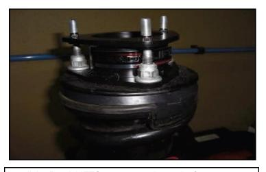
Install the ReadyLIFT $\otimes$  strut extension to the factory strut using factory hardware. Torque to 25 ft-lbs.
