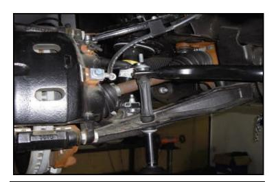
Remove the sway bar end link from the lower control arm
