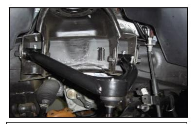
Install the new upper control arms to the frame using factory hardware in the same orientation as removed. Do not tighten at this time.
