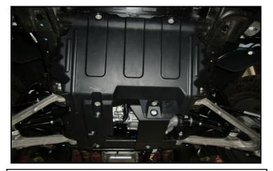
Install the gravel guard using factory hardware on/in the original frame and bracket, and provided M6 x 20mm bolt, washers and nut. Torque to 5 ft-lbs. Make sure to not over tighten and strip out the frame holes. These are self tapping bolts
