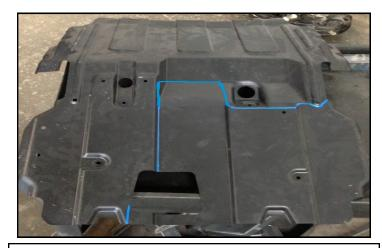
The factory gravel guard will need to be trimmed to fit back onto the vehicle. Mark the gravel guard as shown and use a suitable cutting device, trim the plastic as shown. This is a guide and you may need to trim more after test fitting.
