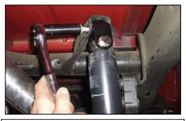
Install the provided shock extension to the frame using factory hardware. Install the factory shock to the extension using M14 x 75mm bolts, washers, and nuts. Install the lower shock to the axle using factory hardware. Do not tighten at this time.
