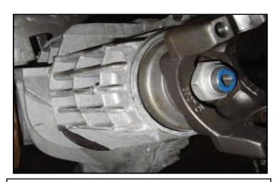
Mark the lowest cooling fin as shown, use a suitable cutting tool, remove the fin. This is for clearance against the driver side rear control arm pocket.
