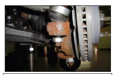
Install the outer tie rod to the knuckle using factory hardware. Torque to 65 ft-lbs.
