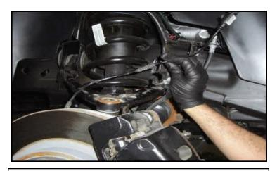
Support the lower control arm with a suitable jack. Loosen but do not remove the lower control arm bolts. Disconnect the ABS connector at the frame. Remove the brake line bracket on the upper control arm.
