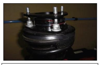
Install the new strut extension to the factory strut using factory hardware. Torque to 25 ft-lbs.
