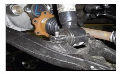
Remove the lower nut clips from the strut. Install the completed strut assembly into the vehicle using M10 flange nuts at the frame and M10 X 60mm bolts, washers, and nuts for the lower control arm. Do not tighten at this time.
