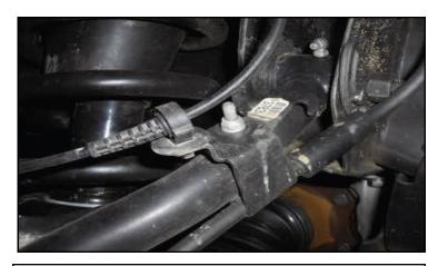
Install the brake line bracket to the control arm using M6 nut and washer. Torque to 5 ft-lbs.
