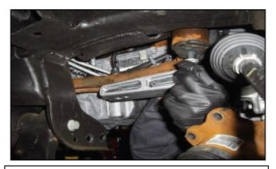
Install the provided passenger differential drop to the hanger using M12 x 80mm (front) and 70mm (rear) socket head bolts and flange nuts. Install the hanger back into the frame using factory hardware. Torque all to 45 ft-lbs.
