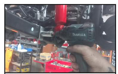
Remove the brake line bracket at the axle.
