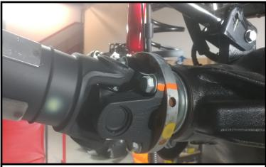
Mark the front drive shaft to pinion. Remove the drive shaft from the pinion. Let hang out of the way.
