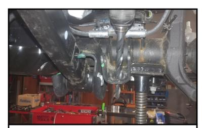
Drill out the lower hole in the shock mount to 1/2".
