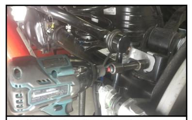
Install the rear bake line to the axle
