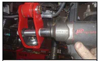
Install the shock to the shock extension using the provided 1/2" hardware. Install the provided crush sleeve and factory hardware. Tighten all.
