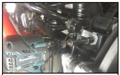
Rear install: Support the axle with a jack. Remove the wheels. Remove the brake line brackets at the axle.
