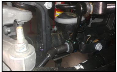
Remove the lower sway bar end links from the axle.
