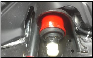
Install the front spring spacer. Then reinstall the factory isolator.
