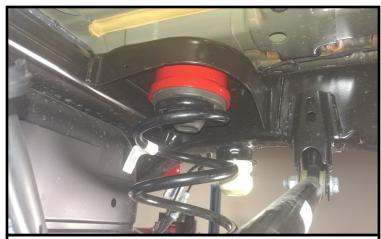
Install the spring and isolator onto the axle and spring spacer. Raise the axle enough to hold all in place.
