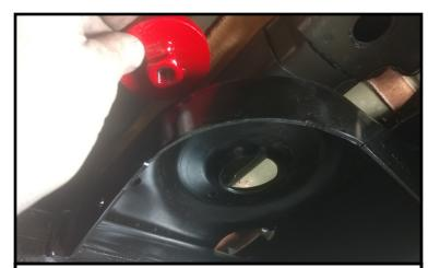
Install the provided nut plate on top of the spring tower.
