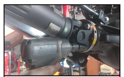
Install the front drive shaft to the pinion using the previously made marks and factory hardware. Use thread locker and tighten.
