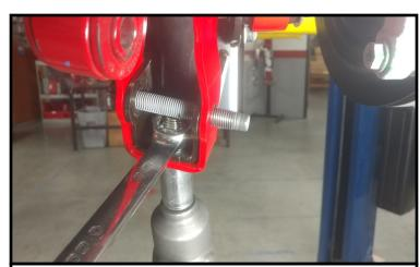
Install the shock extension using the provided 1/2" hardware. Use the factory hardware as a guide. Only tighten the 1/2" hardware now.
