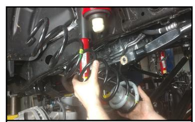
Install the bump stop extension into the spring. Install the spring and bump stop to the axle and frame.
