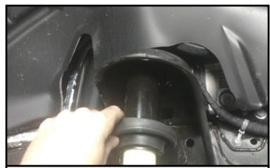
Lower the axle enough to remove the springs and factory isolator.
