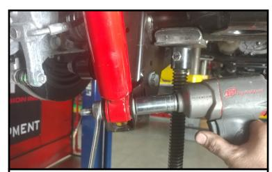
Remove the lower shock from the axle.
