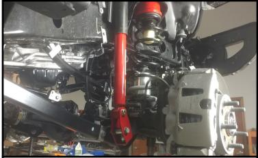
Install the brake line brackets to the frame and control arm using the factory hardware.
