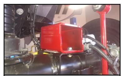
Install the rear bump stop extensions using the provided hardware. Install the wheels and lower the vehicle to the ground. Have the align set.
