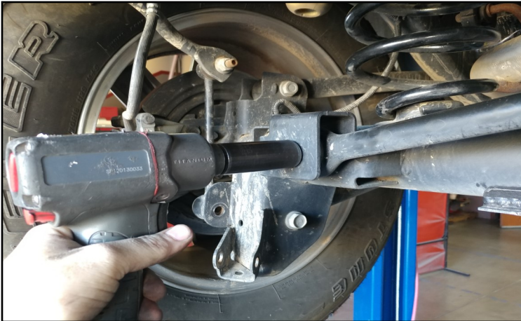
Loosen the track bar at the axle and frame.
