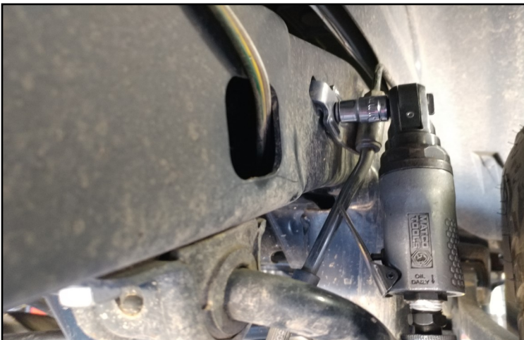
Remove the brake line brackets from the frame.
