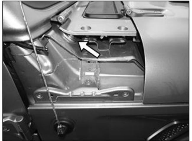
(Fig 4) Remove factory bolts to remove corner body panel. Remove outer bolt from windshield hinge (arrow)
