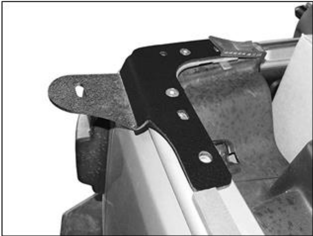
(Fig 12) Passenger/right Mounting Bracket installed
