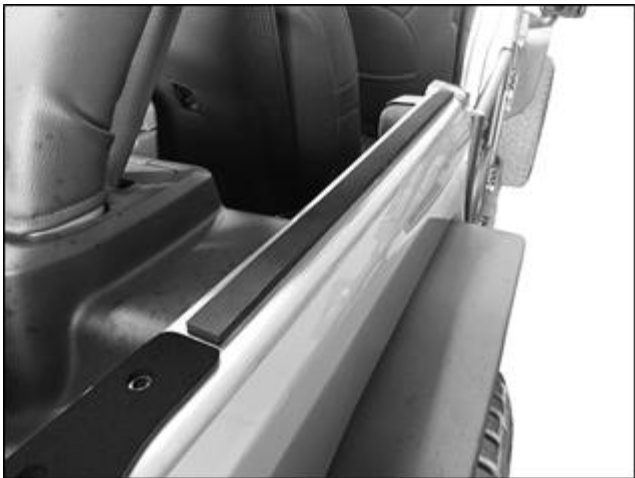
(Fig 14) Install Foam Seal in original location (Shown on 4-door model for example)
