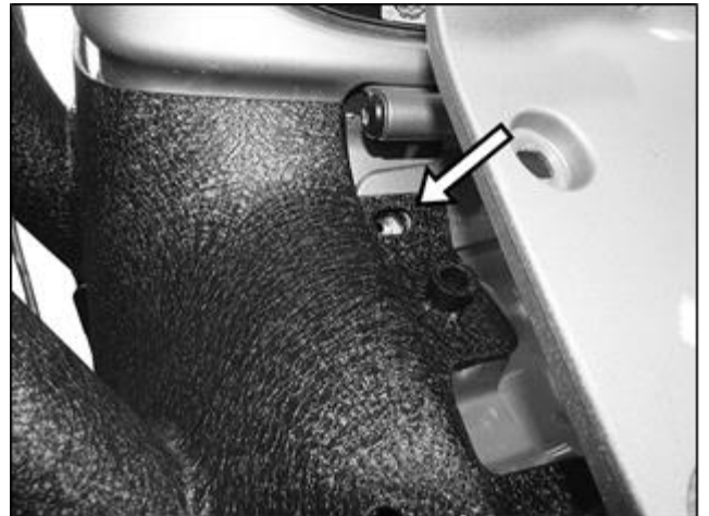
(Fig 6) Reuse factory bolt to attach passenger/right Front Rack Leg to top of windshield hinge
