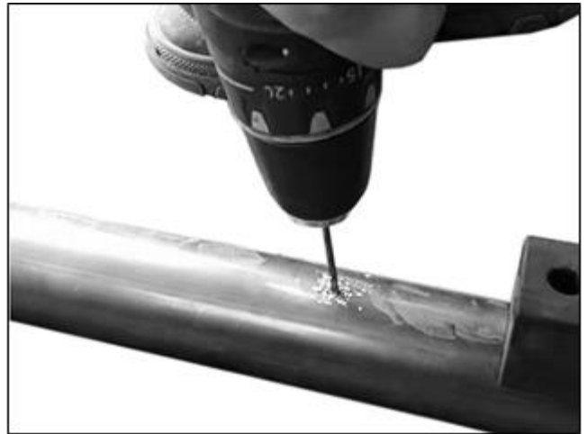
(Fig 22) Drill 1/8" pilot hole
