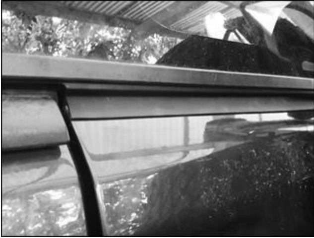
(Fig 27A) Slide Seal over top of tailgate and Tape. Start at end, pull back outer lip on Seal to expose Tape. Slowly remove/pull off outer backing from Tape and stick Seal to Tape and tailgate. Repeat to remove backing from inner Tape on tailgate
