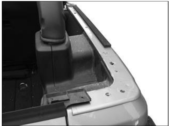
(Fig 10) Passenger/right rear mounting location. Remove factory side to top seal (Shown on 4-door model for example)
