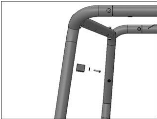
(Fig 23) Attach Bumpers with included #5 Screw and 5mm Flat Washer
