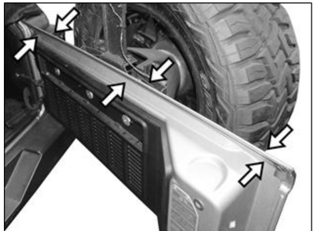
(Fig 24) Clean top of tailgate, inside and outside with included Adhesive Activator
