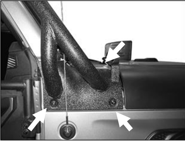
(Fig 7) Reuse factory bolts to attach passenger/right Front Rack Leg to body (arrows). Accessory light not included
