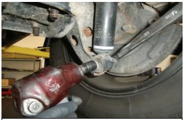
Support the rear axle. Remove the rear shocks, brake line brackets, and parking brake cable brackets from the axle.
