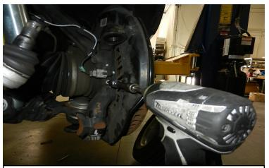
Remove the cotter pin and outer tie rod end nut. Strike the tie rod end boss with a dead blow hammer to dislodge the taper. Remove the ABS sensor and harness from the knuckle and hang out of the way.
