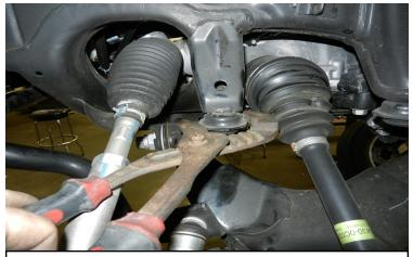
Remove the lower control arm bump stops.
