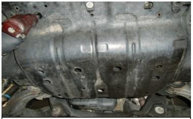
4WD steps: Remove the factory skid plate.
