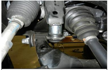
Install the provided bump stop extensions to the frame and the bump stops to the extensions.
