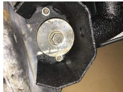
Link the Rocker Panel Guard with the vehicle body, then mount the nut.
