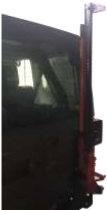
Place the jack on mounting bracket and fixed with under mounting plate, handle nut and Non-slip gasket.
