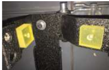
Install the block rubber on mounting bracket and upper mounting plate with Round head bolt of a cross and nut, respectively.
