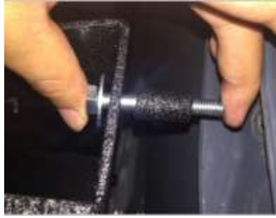
Connect mounting bracket with the car body and tighten with one outside hexagon bolt, M10 flat washer and one circular tube.
