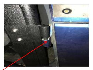
3. Fix the door and Debugging screws.
