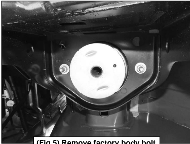
(Fig 5) Remove factory body bolt
