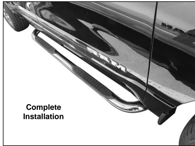
(Fig 12) Driver/left Front Brackets and Sidebar installed
