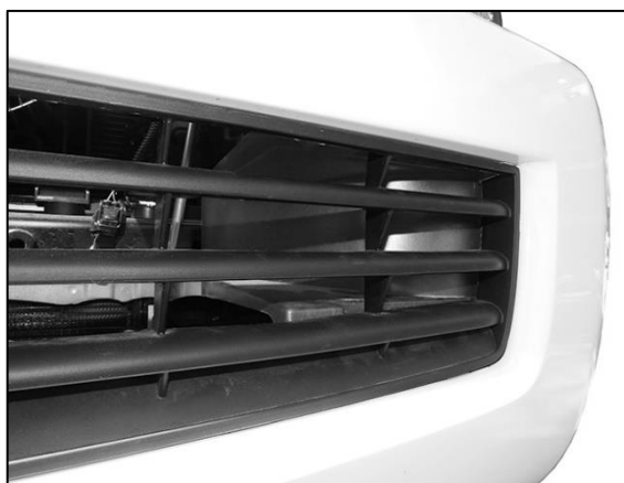
(Fig 5A) Remove or cut air deflector from behind lower grille opening in bumper
