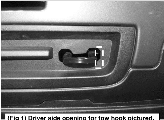
(Fig 1) Driver side opening for tow hook pictured. Dashed white line represents approximate area to cut for Bracket clearance. Check before cutting
