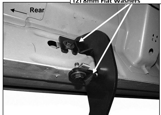
(Fig 7) Driver/left rear bracket installed
