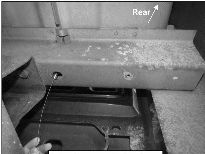
(Fig 6) Insert coiled end of Fish Wire into oval hole
