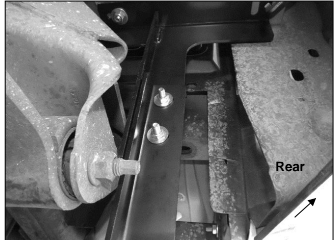
(Fig 16) Passenger side Front Box Board Installed
