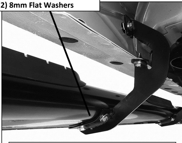
(Fig 21) Passenger side installation pictured
