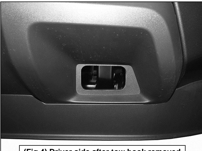
(Fig 4) Driver side after tow hook removed
