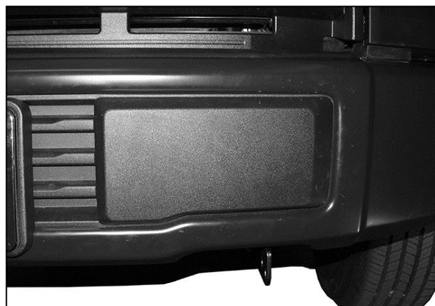
(Fig 6) Remove bumper pads to access splash guard hardware if necessary. 2015 F150 pictured
