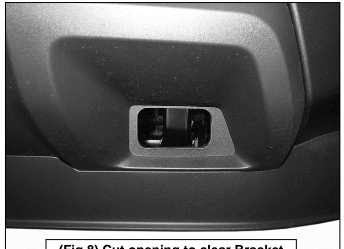
(Fig 8) Cut opening to clear Bracket
