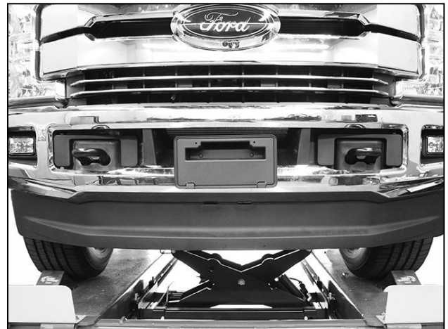
(Fig 6) Remove plastic air dam from bumper
