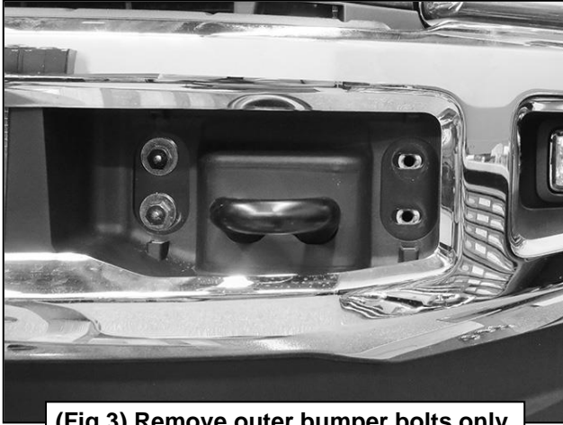
(Fig 3) Remove outer bumper bolts only
