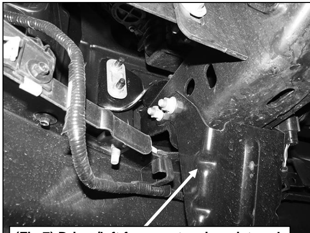
(Fig 7) Driver/left frame extension pictured
