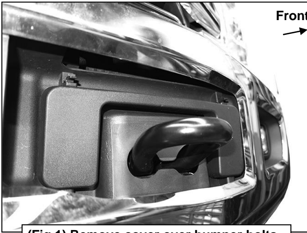
(Fig 1) Remove cover over bumper bolts (2017-19 model year pictured)
