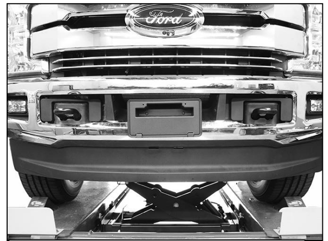
(Fig 6) Remove plastic air dam from bumper
