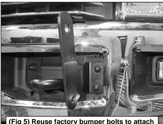
(Fig 5) Reuse factory bumper bolts to attach driver/left Frame Bracket to bumper
