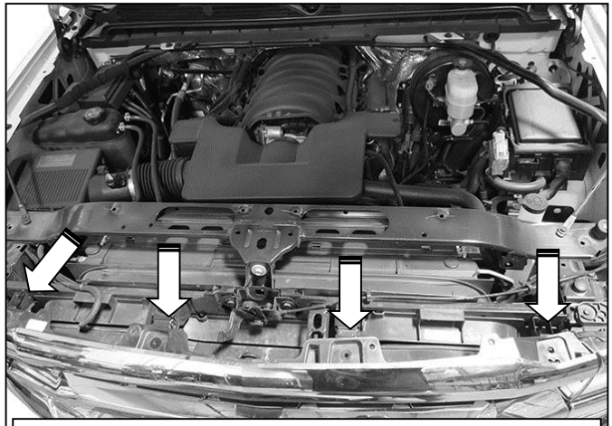
(Fig 2) Remove cover between radiator and grille. Remove screws attaching top of grille (arrows)
