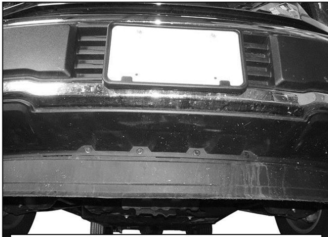
(Fig 1) Remove spoiler and pads from bumper
