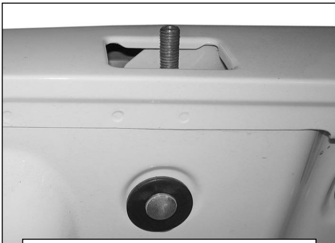
(Fig 5) Use the 10mm J-Bolt to secure the front mounting holes on the Bracket to the stake pocket if possible. Do not drill any mounting holes until after all mounting locations are checked for clearance
