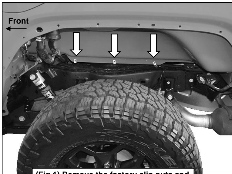
(Fig 1) Remove the factory clip nuts and slide (3) 6mm Clip Nuts onto the (3) mounting holes inside the wheel well
