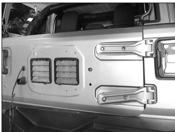
(Fig 7) Remove hardware attaching outer hinges to tailgate. NOTE: Bolts are tight, clean sockets on screws before inserting Torx tool
