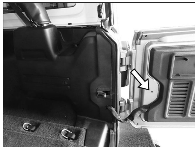
(Fig 2) Remove the bolt attaching the check rod to the tailgate. Push check rod in, remove plastic covers from right side of cargo area and tailgate
