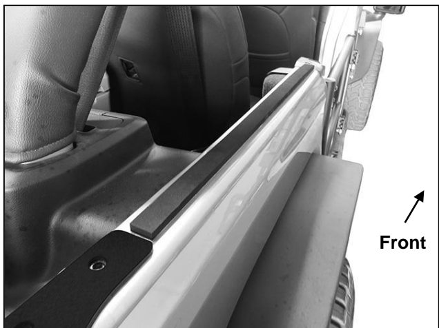
(Fig 16) Install Foam Seal in original location
