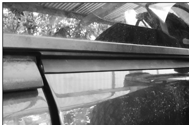
(Fig 26A) Slide Seal over top of tailgate and Tape. Start at end, pull back outer lip on Seal to expose Tape. Slowly remove/pull off outer backing from Tape and stick Seal to Tape and tailgate. Repeat to remove backing from inner Tape on tailgate
