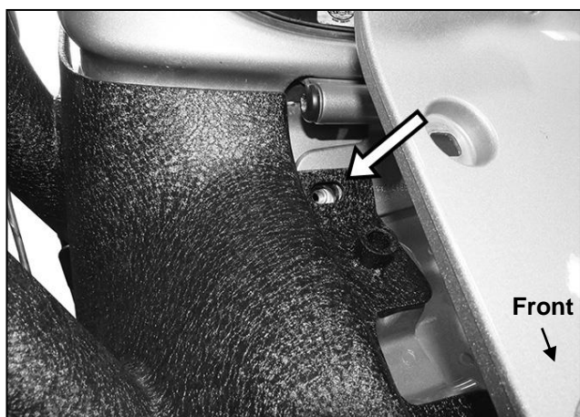
(Fig 7) Reuse factory bolt to attach passenger/right Front Rack Leg to top of windshield hinge
