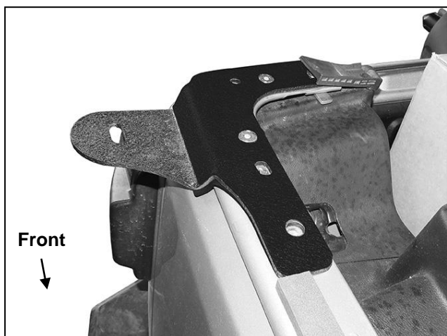
(Fig 14) Passenger/right Mounting Bracket installed
