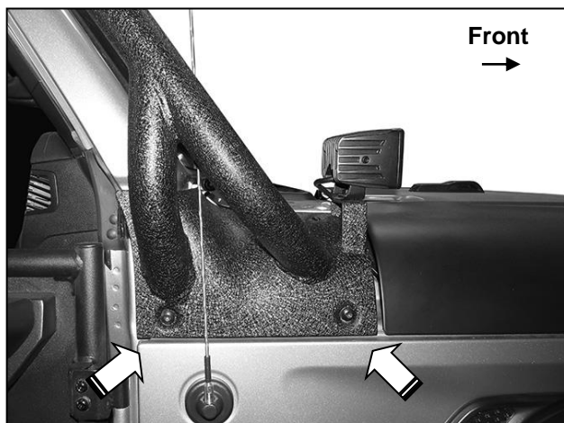
(Fig 8) Reuse factory bolts to attach side of passenger/right Front Rack Leg to outside of body (arrows). Accessory light not included
