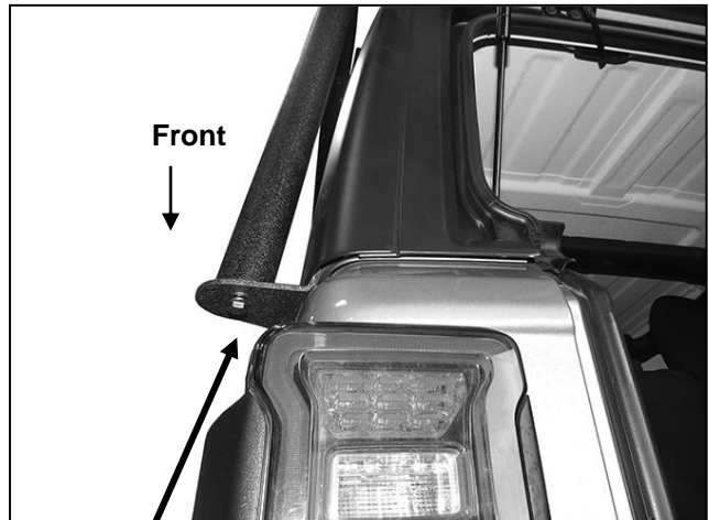
(Fig 22) Rear Leg attached to Mounting Bracket (driver/left side pictured)
