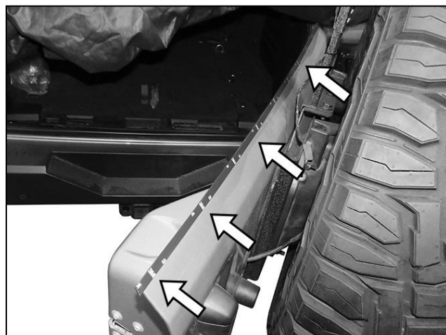
(Fig 24) Apply (1) strip of Double Sided Tape to outside of tailgate, DO NOT REMOVE OUTER BACKING TAPE! Repeat to apply (1) strip of Tape to inside of tailgate
