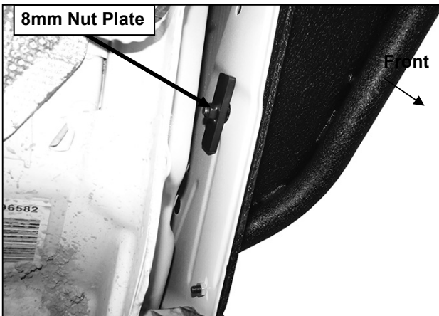
(Fig 7) Slide 8mm Nut Plate behind mounting hole in body panel. Attach Fender to Nut Plate (Fig 6)
