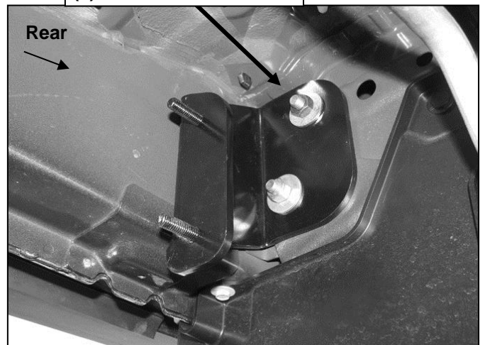
(Fig 24) Passenger rear Frame Bracket installation
