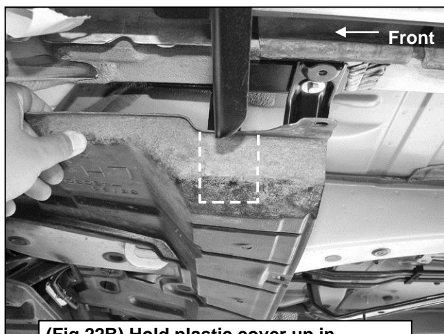
(Fig 22B) Hold plastic cover up in position to determine area to cut from cover. Driver side front cover pictured
