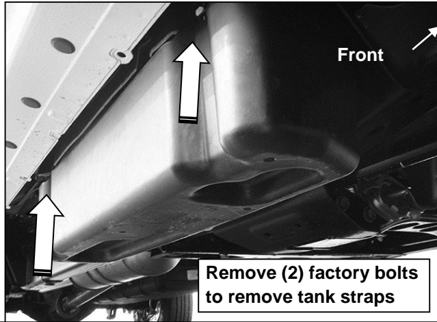
(Fig 13) 07-16 Passenger side DEF tank and cover
