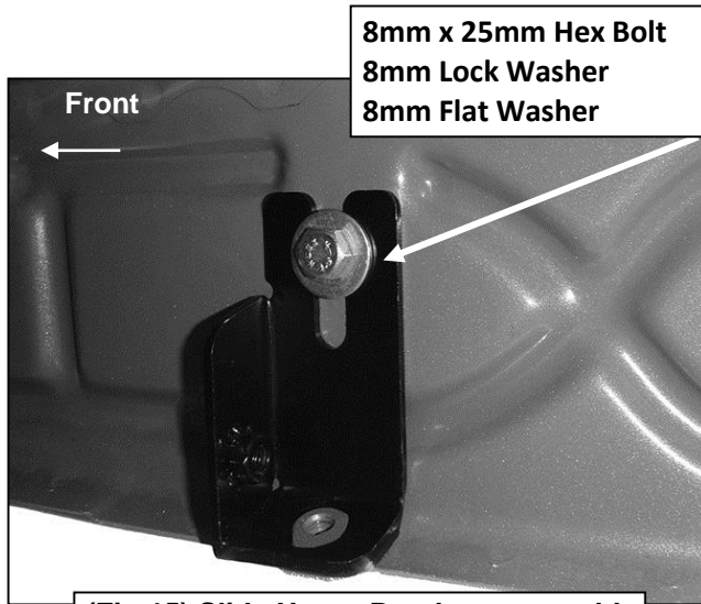
(Fig 15) Slide Upper Bracket over weld nut if equipped-also see Figure 2
