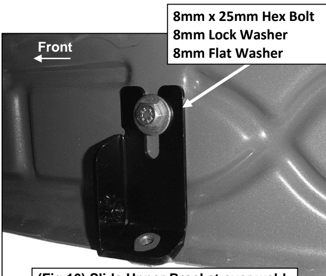
(Fig 16) Slide Upper Bracket over weld nut if equipped-also see Figure 2
