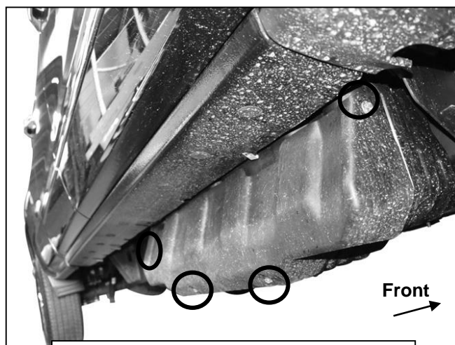
(Fig 13A) 2017 Passenger side pictured with DEF plastic tank cover. Remove (4) hex bolts to remove plastic cover
