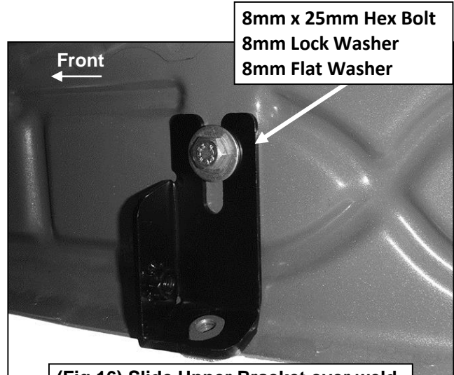
(Fig 16) Slide Upper Bracket over weld nut if equipped-also see Figure 2
