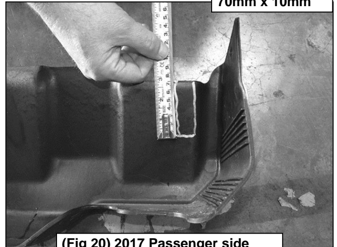
(Fig 20) 2017 Passenger side DEF cover marked for trimming
