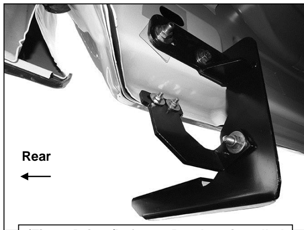
(Fig 17) Driver/Left rear Brackets installed
