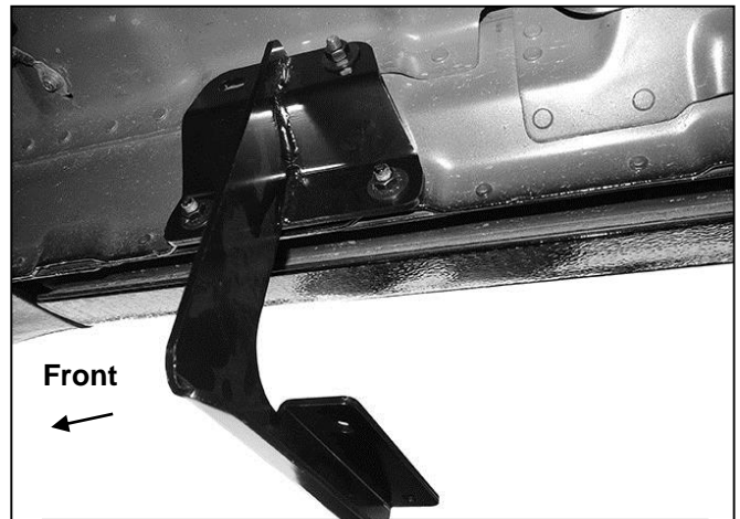
(Fig 5) Passenger/right front Bracket installed
