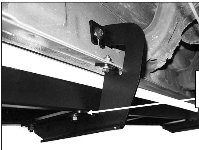
(Fig 12) Driver/left rear Running Board to Bracket
