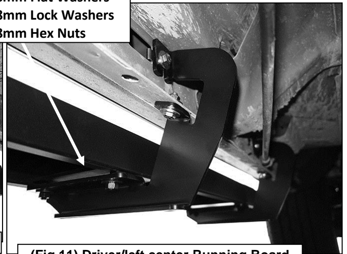
(Fig 11) Driver/left center Running Board to Bracket
