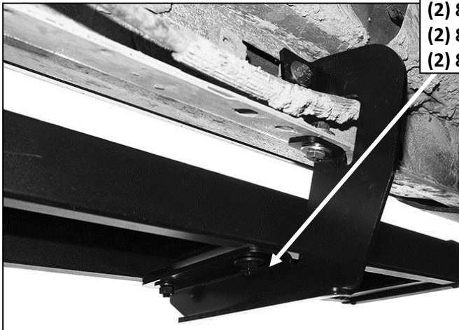
(Fig 10) Driver/left front Running Board to Bracket
