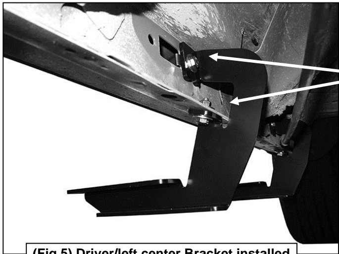
(Fig 5) Driver/left center Bracket installed
